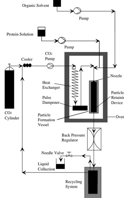
**Figure 1.** Schematic diagram of the SEDS experimental set-up.
